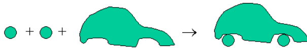
Fig. 4.3 Production of automobiles requires the ordering of many parts: screws, nuts and bolts, wires, tires, wheels etc. All parts have to be placed in the correct position and in the right order, the entropy is reduced, d F < 0 .
