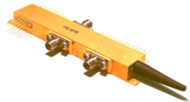
Figure 2. DQPSK transmitter module containing GaAs encoder together with DFB laser source.
