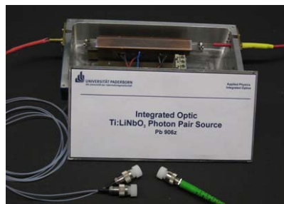
Fig. 2: Photograph of the packaged photon pair source.
