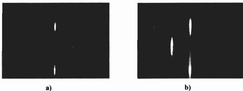
Fig.1 RHEED pattern of the InGaN growth,
